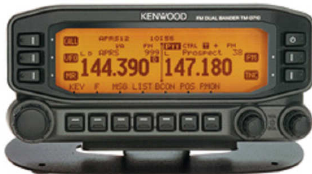
Figure 1 — Here, the TM-D710A's control head is set up for APRS operation on the left side and voice operation on the right.
